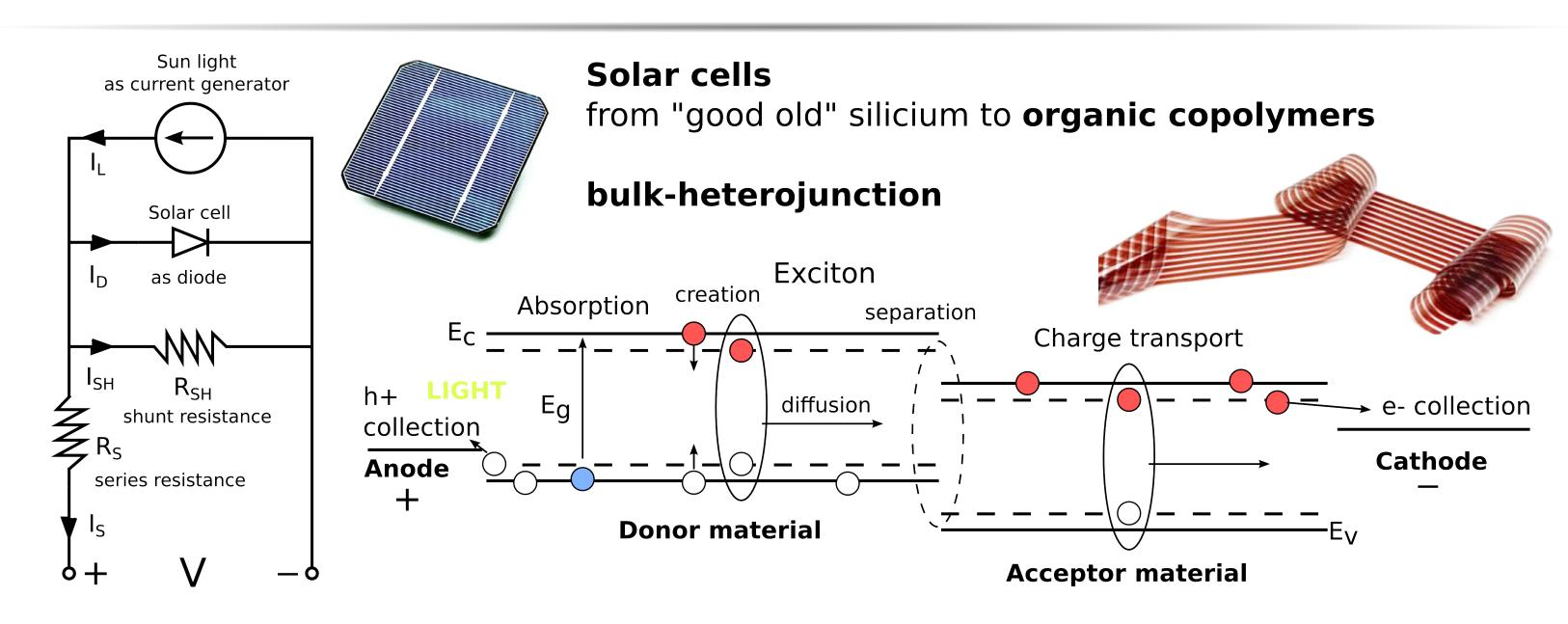
We choose hybrid organic solar cells because of the possibilities that are added with the use of **organic polymers**. The advantages that this new technology offers are:
