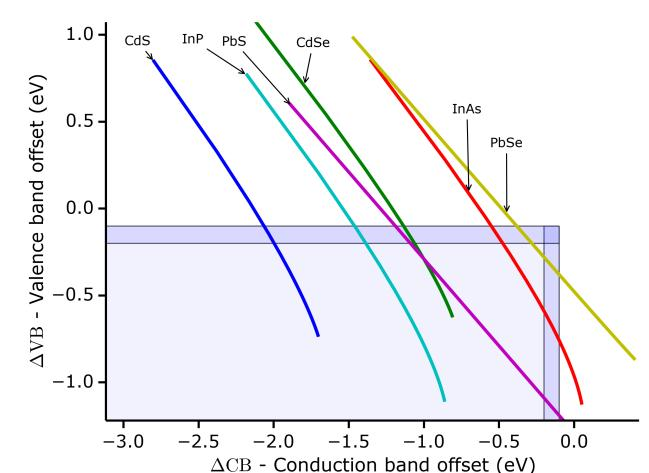
Best acceptor for **PDPP2FT** = PbSe (tested) QDs band-edges for sizes between 1 and 20 nm. Search window:  $\Delta CB$  et  $\Delta VB$  between -0.1 and -0.2 eV or less.
